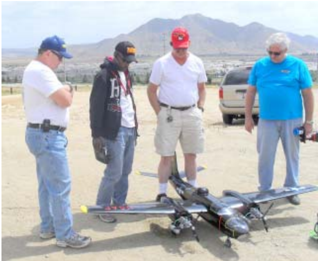
Discussing the flight plan for the as-yet unflown A-26 Bomber. Powered by two Magnum .91 4-strokes, it is expected to be very fast.
